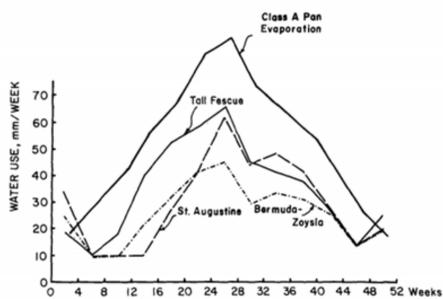
Fig. 3. Seasonal pattern of consumptive use for tall fescue, St. Augustinegrass and bermudagrass-zoysiagrass under low management compared with Class A pan evaporation.
